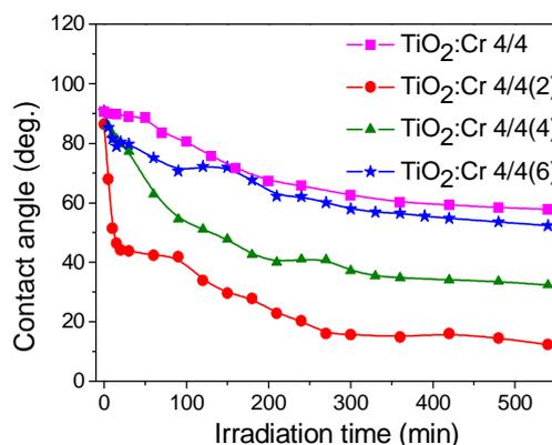
**Fig. 3.8** Contact angle as a function of the irradiation time for the TiO<sub>2</sub> films with the highest Cr concentration (TiO<sub>2</sub>:Cr 4/4), having different Pt islands deposited on their surfaces
