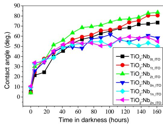
**Fig.3.5** Contact angle versus time dependences, as monitored during the back-reaction regime
