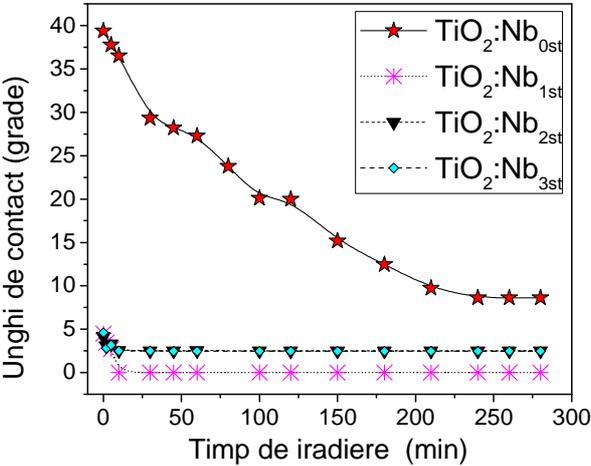
Fig. 3.1 Contact angle vs. UV irradiation time plots for the pristine TiO<sub>2</sub> and TiO<sub>2</sub>/Nb samples
