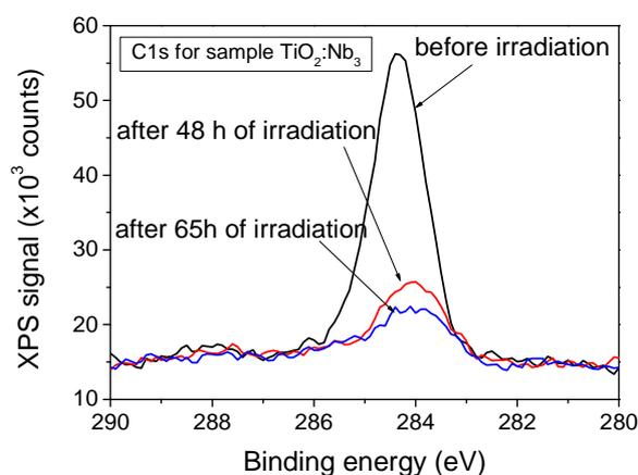
**Fig. 3.6** C 1s XPS spectra of the film S3 covered with oleic acid, before the UV irradiation, and after 50 hours and 65 hours after irradiation
