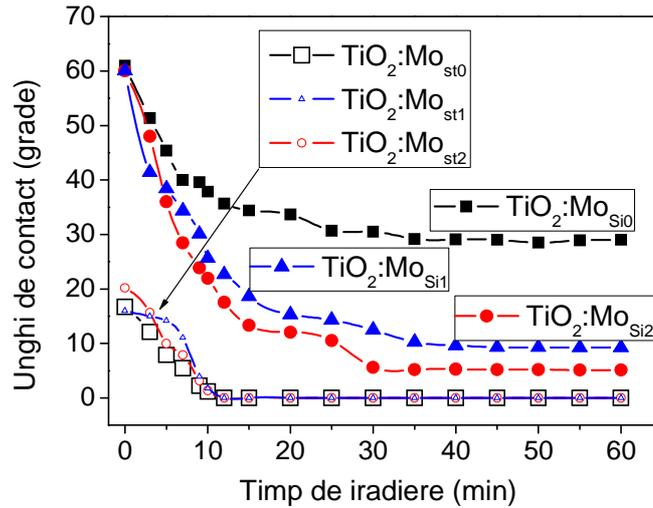
**Fig. 3.7** Contact angle as a function of the irradiation time for all the studied samples [Adomnitei et al. 2014]
