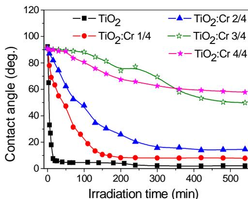
**Fig. 3.7** Contact angle as a function of the irradiation time for the TiO<sub>2</sub> films having different Cr percentages
