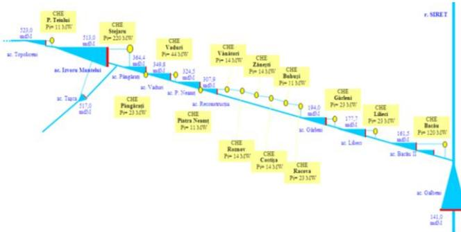
Fig. 1 Bistrița River Hydropower development (source Siret Water Basin Administration, 2015)
