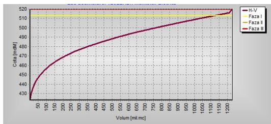
Fig. 2 Volumetric curve of IZVORU MUNTELUI Reservoir
