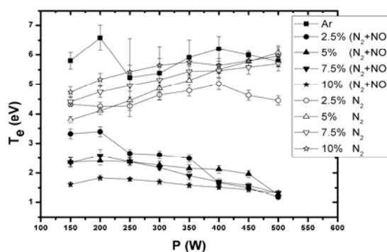
Fig.10. Changes in power of electron temperature measured with the triple probe in Ar plasma in which different concentrations of  $N_2$  and  $N_2 + NO$  were added [33]
