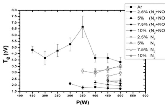
Fig.9. Changes in power of electron temperature measured with the single probe in Ar plasma in which different concentrations of  $N_2$  and  $N_2 + NO$  were added [42]
