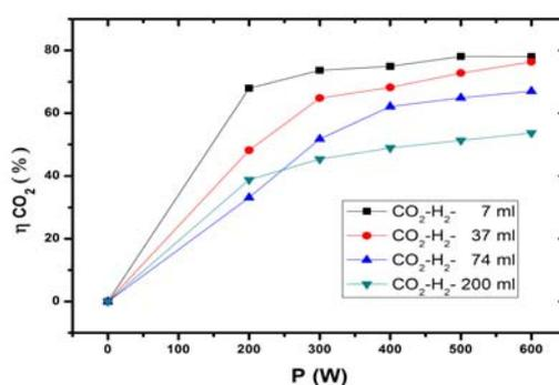
Fig.6. The yield of  $\text{CO}_2$  dissociation in a microwave plasma where the microwave radiation power and the flow of  $\text{CO}_2$  and  $\text{H}_2$  introduced varied
