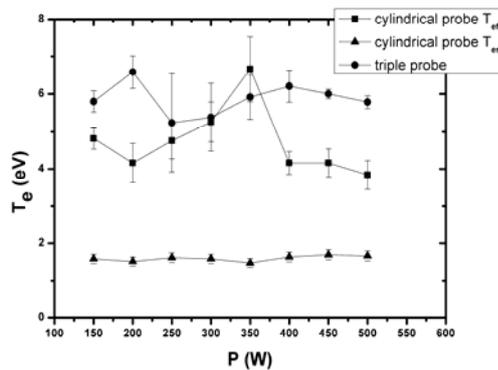
Fig.8. Electron temperatures measured with a simple probe and triple probe in Ar microwave plasma [42]
