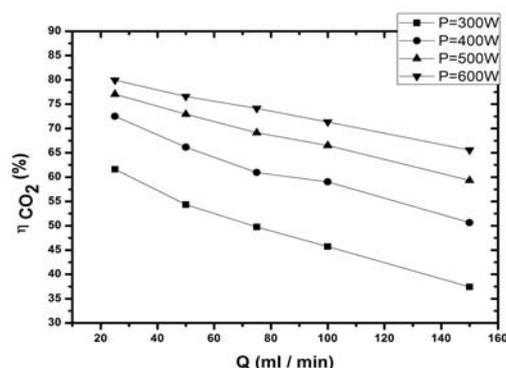
*Fig.7. The yield of CO<sub>2</sub> dissociation in a microwave plasma where the microwave radiation power and the flow of CO<sub>2</sub> introduced varied, for a stable pressure of 2.1 Torr*
