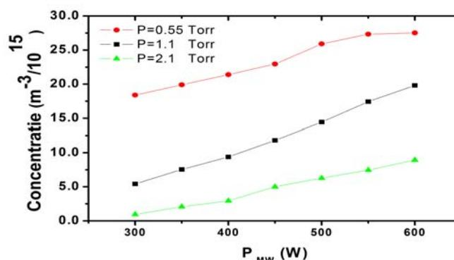
*Fig.4. Changes in the concentrations of metastable oxygen atoms in relation to the microwave radiation power and the working gas pressure*
