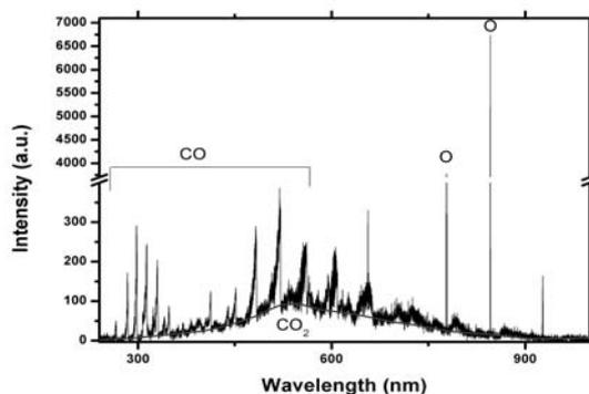
Fig.2. The emission spectrum of a CO<sub>2</sub> microwave plasma discharge
