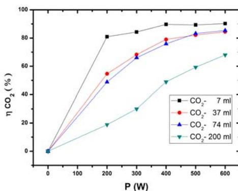
Fig.5. The yield of  $\text{CO}_2$  dissociation in a microwave plasma where the microwave radiation power and the flow of  $\text{CO}_2$  introduced varied
