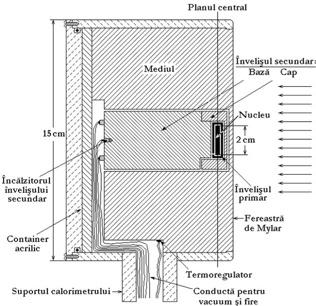
**Fig. 4.** Section via the NBS graphite calorimeter (and/or ENEA-INMRI), side view [15, 76]
