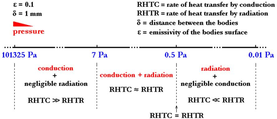
Fig. 6: Diagram of the connection between the air pressure value and the dominant phenomenon via which the heat transfer takes place
