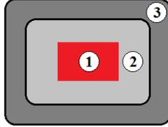
**Fig. 2:** The main parts of a calorimeter: 1-the thermally active body (or absorbent); 2 - the thermally isolating medium; 3 - the jacket
