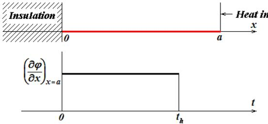
**Fig. 10:** Graphic representation of the extreme conditions for the one-dimensional model
