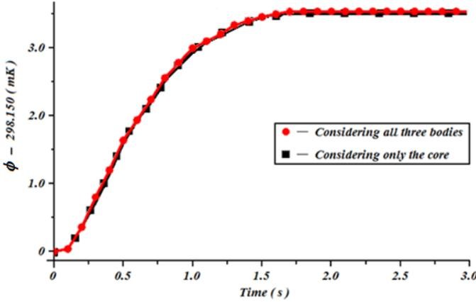
**Fig. 12:** The increase in temperature of the core based on time, measured from the beginning of the core's heating, in two cases: (i) the 3D numerical analysis of the entire calorimeter (considering all three interior bodies of the calorimeter) – the red curve (the dotted curve) and (ii) the 3D numerical analysis of the nucleus only – the black curve (the square curve)
