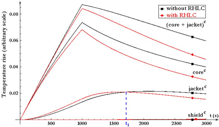
**Fig. 7.** Variation in temperature increase of the three bodies on the inside of the graphite calorimeter, with RHLC (red curves) and without RHLC (black curves), for  $t_h = 1000$  s heating
