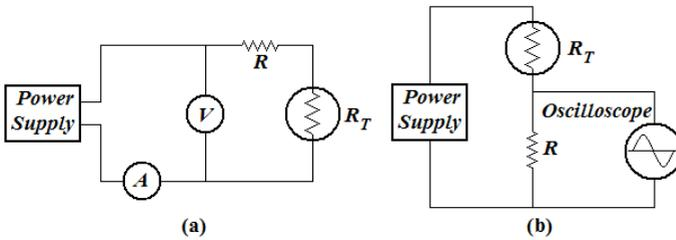
**Fig. 5:** Testing circuits (a) for the measurement of dissipation constants and (b) for the measurement of time thermal constants with low and very low values[93]
