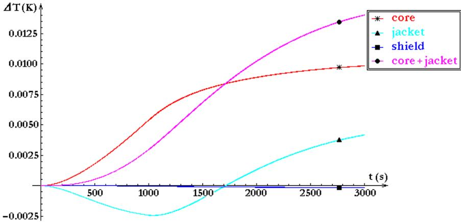
Fig. 8. The  $\Delta T_i = \Delta T_i(t)$ , ( $i=1,4$ ) dependencies for an overall time of 3000 s (1000 s plus 2000 s the heating thermal relaxation)
