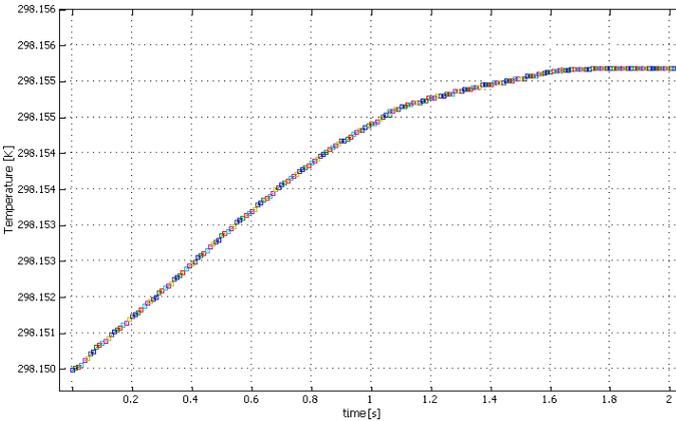
**Fig. 13:** Temporal dependency of the core's temperature in the location points of the sensing thermistor  $s(P_1$  and/or  $P_2$ ) for the first heating  $\Delta t = 2$  s. This is the temperature „measured” by the sensing thermistors.
