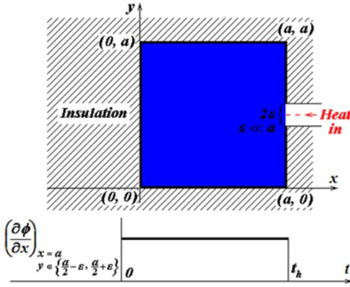
**Fig. 11:** Graphic illustration of the borderline conditions for the equation (\*\*)
