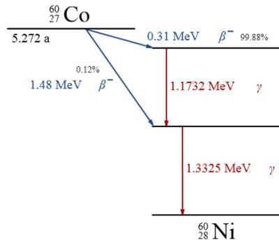
**Fig. 1.** The disintegration diagram of the most used  $\gamma$ -active radionuclide,  $^{60}\text{Co}$  [65]
