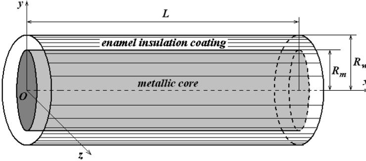
**Fig. 9.** The spatial orientation of the coordinate axes attached to a connection wire of the thermistors:  $R_m$  is the radius of the metallic core of the wire, and  $R_w$  is the overall radius of
