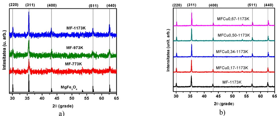
Fig.3.1. MF (magnesium ferrite) and MF doped with Cu nanopowders diffraction patterns treated at different temperatures [6, 7].
