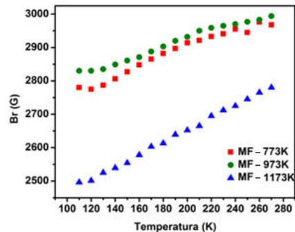
Fig. 4.5. The temperature dependence of the resonance field for MF nanoparticles annealed at different temperatures.
