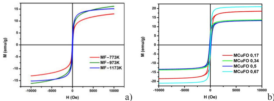
Fig. 4.1. Hysteresis curves of ferrite nanopowders a)Mg, b)Mg doped with Cu [6, 7].
