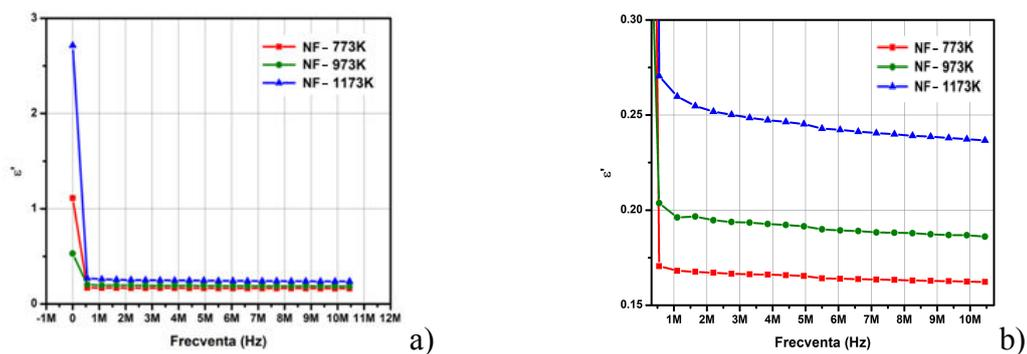
Fig. 4.6. The real part of permittivity ( $\epsilon'$ ) as a function of frequency for thermally treated NF nanoparticles: a) 40Hz – 10,5MHz; b) 0,5MHz – 10,5MHz.
