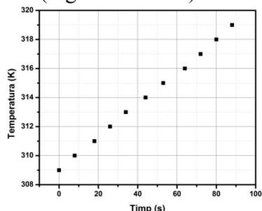
Fig. 4.7. Temperature evolution as a function of time in colloid I (magnetite with PEG).
