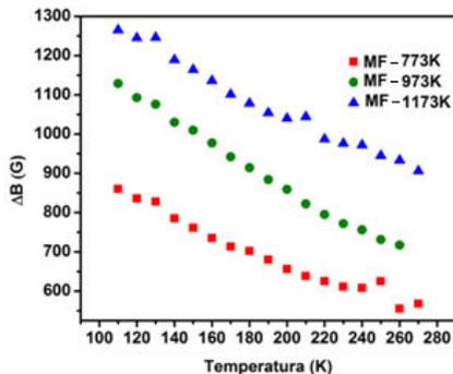
Fig. 4.4 . The temperature dependence of the ESR signal linewidth for MF nanoparticles annealed at different temperatures.
