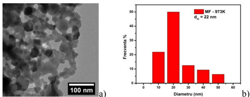
Fig. 3.2. a) TEM micrograph of MF (magnesium ferrite) nanopowders of thermally treated at 973K; b) distribution of MF nanoparticles.
