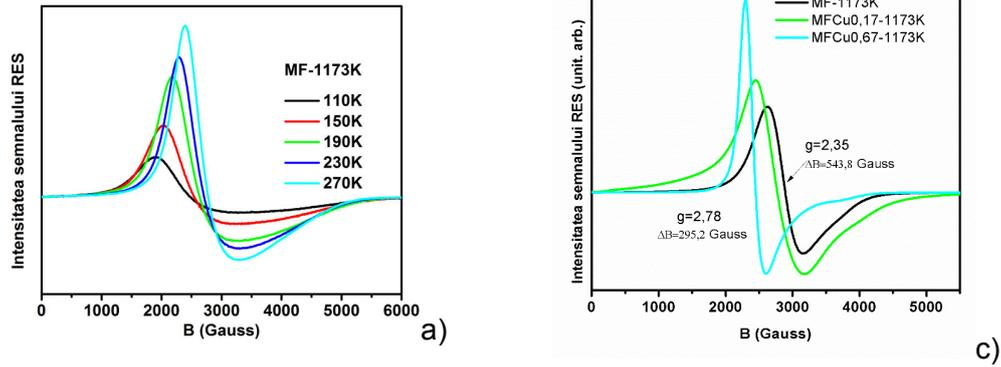
Fig. 4.3. ESR spectra of MF and MF doped with Cu nanopowders depending on the temperature thermally treated at different temperatures [6, 7].
