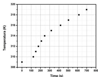
Fig. 4.8. Temperature evolution as a function of time in colloid II (magnetite with MEG).
