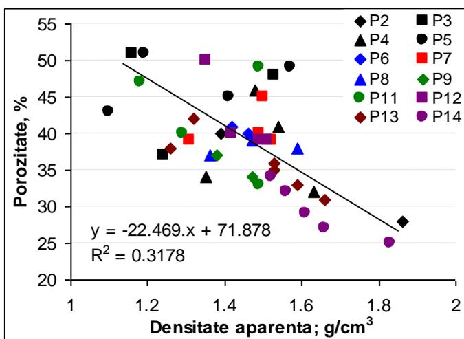
**Figura V.2.** The correlation between porosity and bulk density in the soil from the urban area of Iasi.
