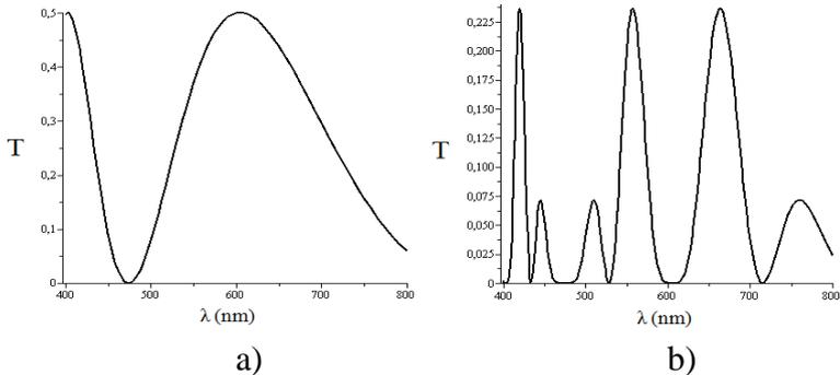
Fig.III.5. The transmission factor of a Lyot filter with a) one layer; b) 3 layers with anisotropic quartz plates(L=100 $\mu$ m)
