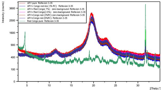
Fig.II.8. Crossed diffractograms of pure PVA samples, of the pure CR and PVA+RC with various concentrations.
