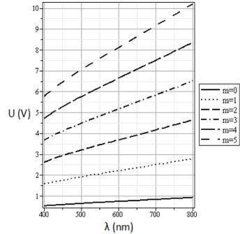
Fig.III.2.The U(V) dependence on  $\lambda$  for  $\lambda/4$  a single layer of PMAECOA ( $L=14\mu\text{m}$ )
