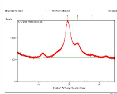
Fig.IV.3. The diffractogram of a PVA foil
