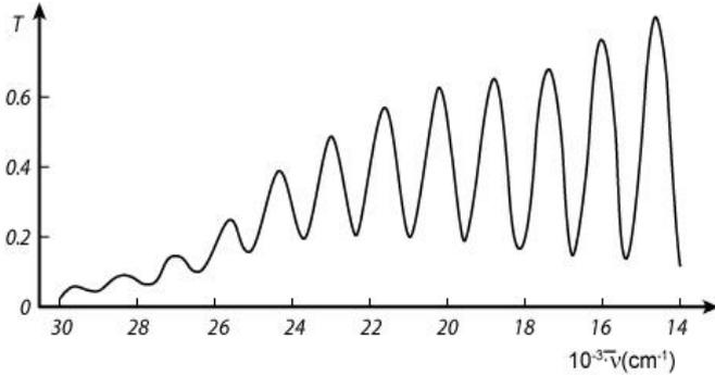
Fig.II.6. Channeled spectra of a natural quartz crystal
