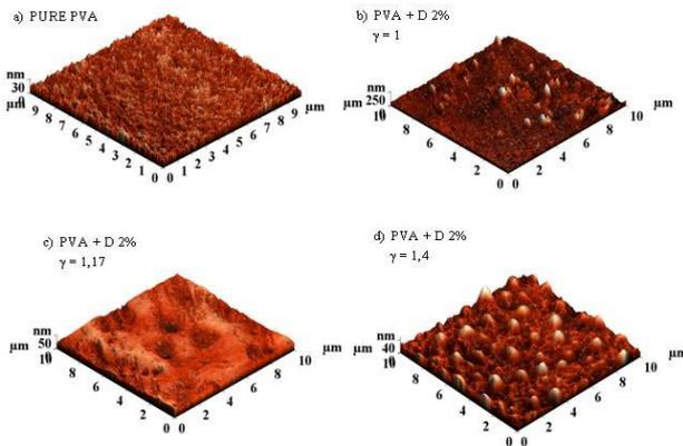
Fig.II.12. AFM images for a) pure PVA; b) PVA+D2% for extended foils ( $\gamma = 1$  ); c) PVA+D2% ( $\gamma=1,17$ ); d) PVA+D2% ( $\gamma=1,4$ )
