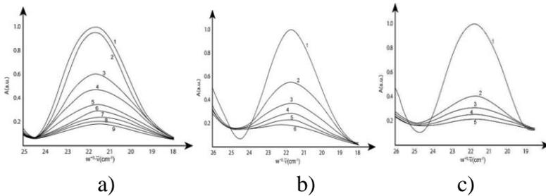
Fig.II.9. The electronic absorption spectra of the ylides: a)CY1; b)CY2; b)CY3.
