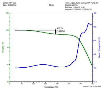
Fig. IV.6. The thermogravimetric analysis for PVA
