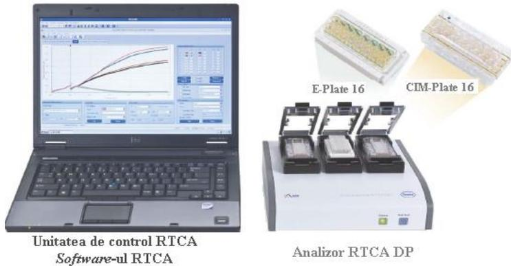
**Fig. 3.** *The RTCA DP instrument with the main components [22].*
