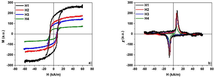
Figure 4.1: The curves  $M = f(H)$  (a) and  $\chi = f(H)$  (b) for H1, H2, H3 and H4 samples [4]
