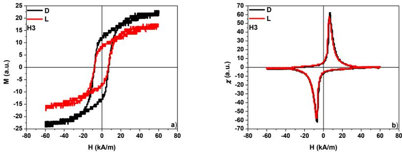
Figure 5.3:  $M = f(H)$  (a) and  $\chi = f(H)$  (b) curves for H3 sample
