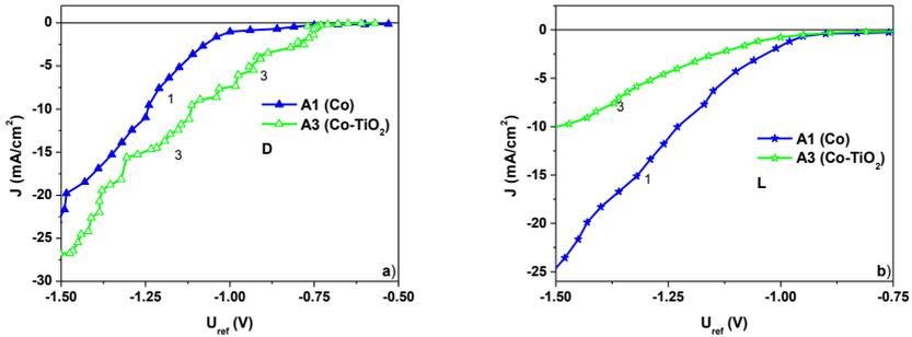
Figure 5.4: The  $J = f(U_{ref})$  curves drawn in the dark (a) and under UV radiation (b) for A1 and A3 samples
