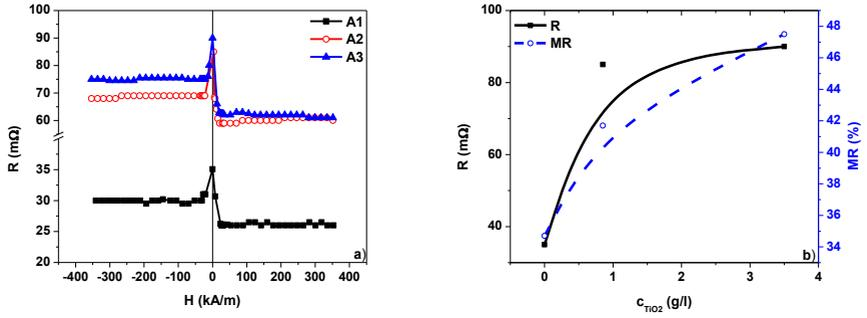
Figure 5.1:  $R = f(H)$  curve (a) and (b)  $R = f(c_{\text{TiO}_2})$  and  $MR = f(c_{\text{TiO}_2})$  curves for A1, A2 and A3 films [1]
