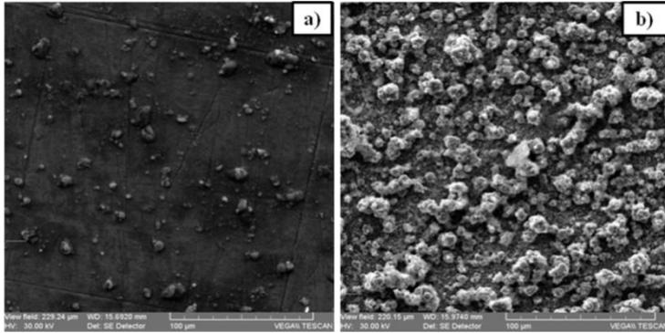
Figure 3.2: SEM micrographs for the films: a) H1 ( $1.1 \text{ A} \cdot \text{dm}^{-2}$ ) and b) H2 ( $3.2 \text{ A} \cdot \text{dm}^{-2}$ ) [4]
