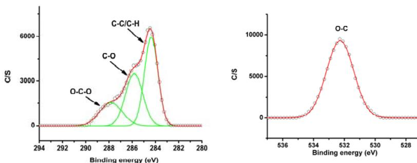
Figure 2.3. Deconvolution of the XPS spectra of ppEG films corresponding to the peak (a) C1s and (b) O1s
