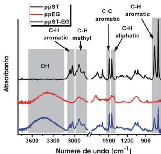
Figure 2.7. FTIR spectra of pST-EG, pST and pEG films obtained by atmospheric pressure plasma polymerization
