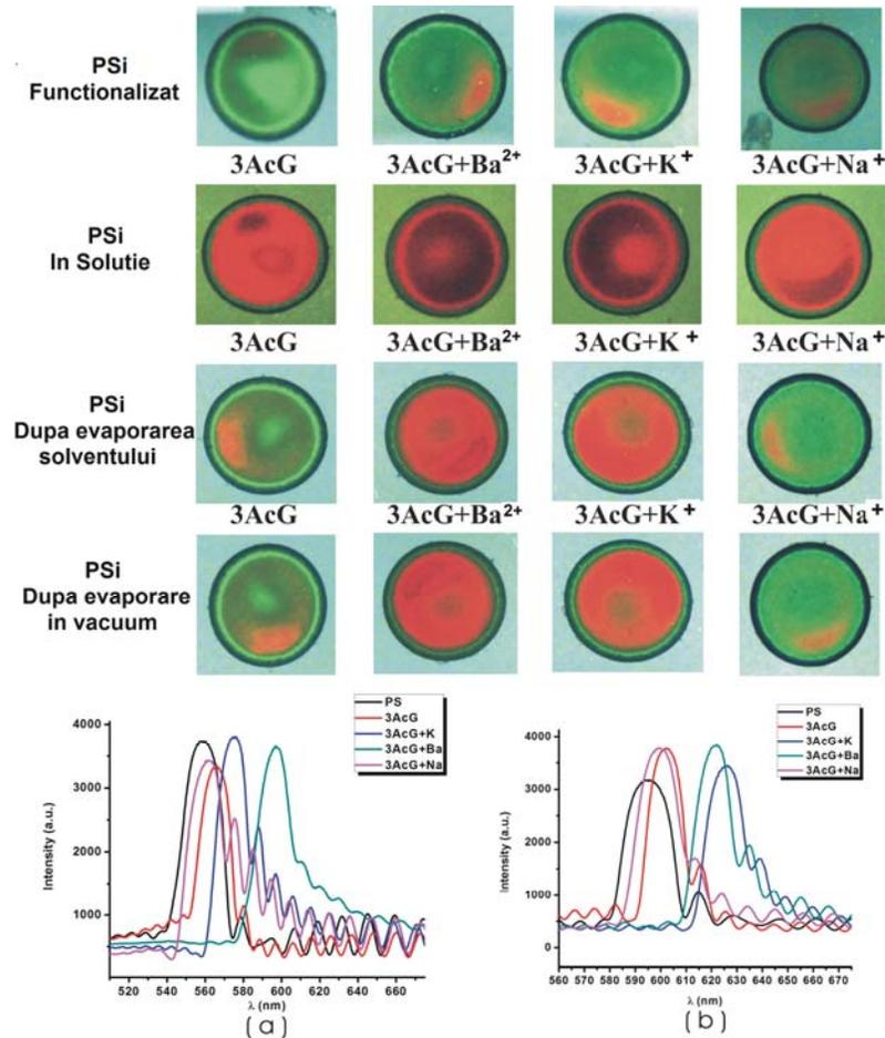
Figure 5.4. Changing in the color of the porous silicon film and the Bragg's "peak" from the reflection spectrum (a) and (b) at the time of their introduction into the liquid solution, and after evaporation of the solvent at room temperature and then in a vacuum conditions
