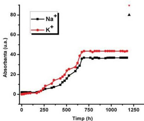
Figure 4.2: Diffusion of ions (Na + and K +) measured using a flame atomic absorption spectrometer through the pores of MCM 41 functionalized with crown ether 15C5
