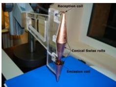
*Figure VI.18 The electromagnetic transducer using metamaterials lens*
