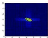
*Figure V.8. Holography imagine of delamination due to an impact with 0.75J energy on the composite taken into study*
