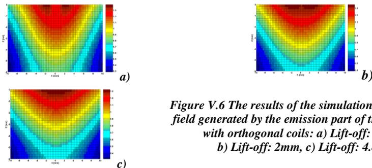
*Figure V.6 The results of the simulation of the electric field generated by the emission part of the transducer with orthogonal coils: a) Lift-off: 0.5mm, b) Lift-off: 2mm, c) Lift-off: 4.8mm*
