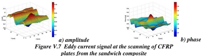
*Figure V.7 Eddy current signal at the scanning of CFRP plates from the sandwich composite*
