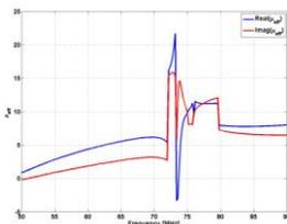
***Figure VI.14 Dependency by frequency of the effective magnetic permeability of conical Swiss roll***
