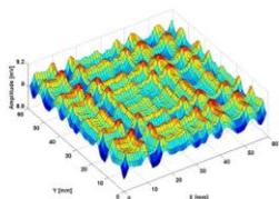
*Amplitude of the signal delivered by the transducer at the scanning of CFRP
